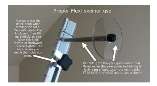
Even though the Flexi-Skeiner is made from steel, we have had one customer that was wrapping their yarn so tightly that they actually bent the bolt inside the stainless steel tube.
